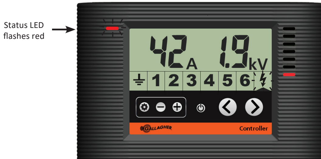
Controller showing the energizer in current alarm
