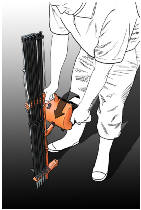
STEP 1 Loosen lock nut (anti-clockwise).
