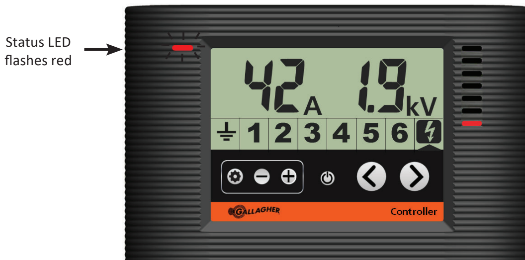
Controller showing the energizer in output alarm
