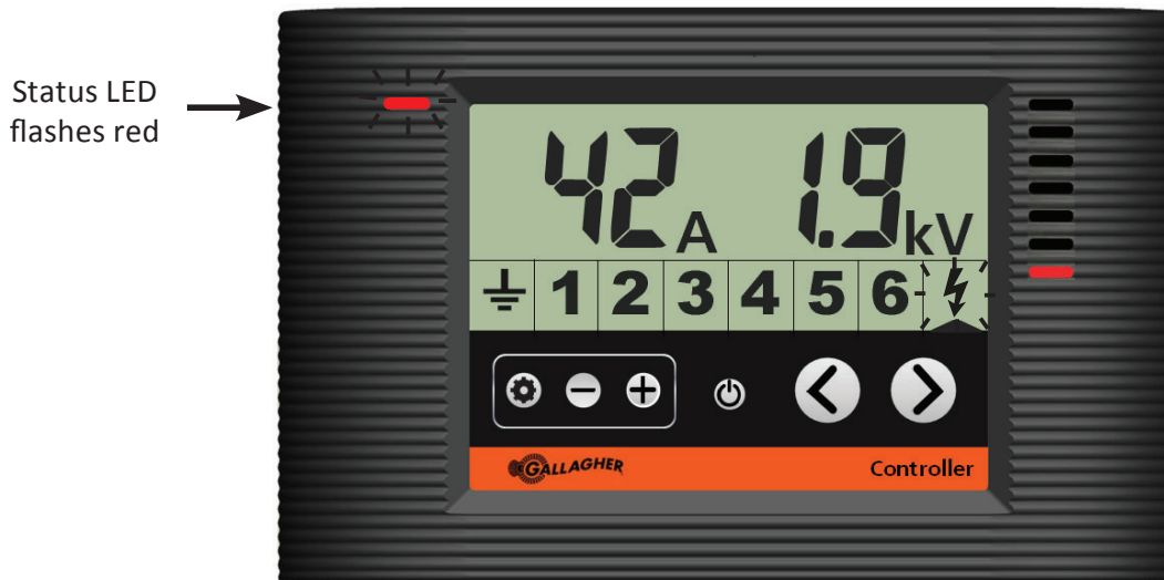
Controller showing the energizer in current alarm
