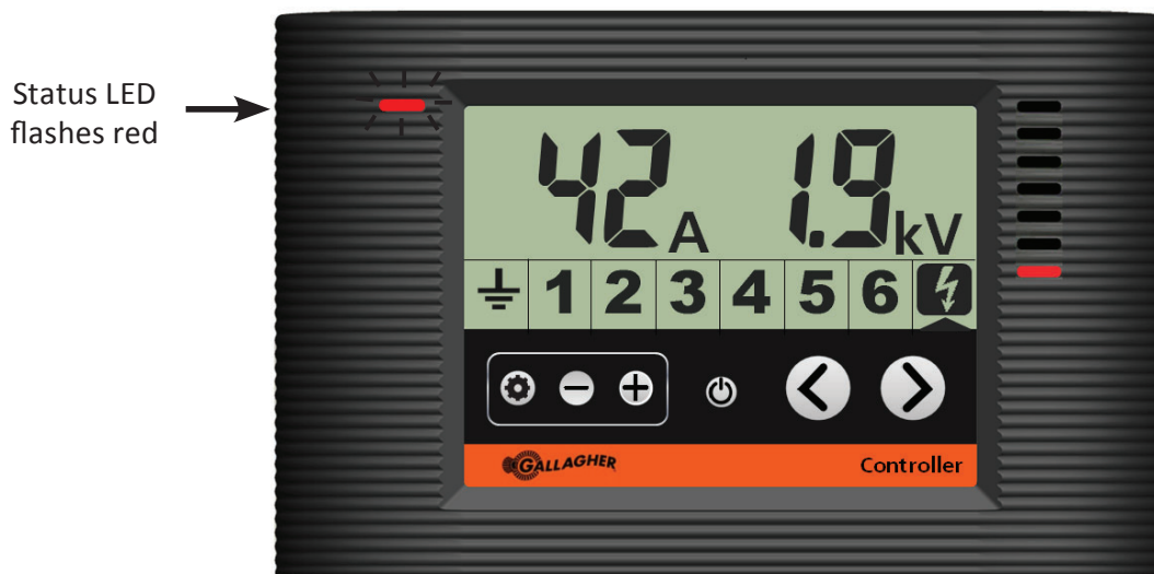
Controller showing the energizer in output alarm
