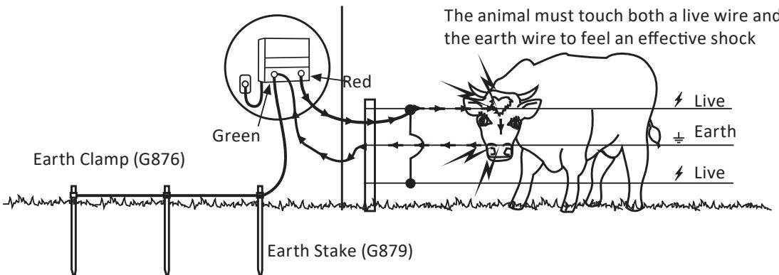
Earth stakes, at least 2m (6ft) long, should be spaced 3m (10ft) apart. Use a minimum of 3 earth stakes for the M600, M700, M1200.
