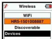
**Note:** For the app to connect to HR4, both devices need to be on the same Wi-Fi access point.
