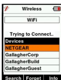
**Note:** The HR4 can be configured to send and/or receive data from other devices via Bluetooth and WiFi.
