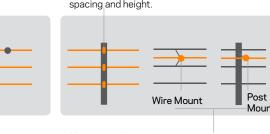
**Offsets** specific to Offset Fencing, hold the electric wire off the existing non-electric fence wire or posts on a conventional fence line.
