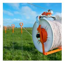
Use an insulated handle on the far end of your portable electric fence so the fence is only powered from one side (at the geared reel). This ensures that the portable fence loses power once you disconnect the alligator clamps and geared reel so you can roll up the wire without getting shocked.
