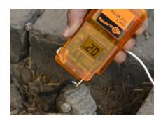
There should be no reading on the Volt Meter; however, up to 200V (0.2kV) is acceptable. If the voltage is higher than this, switch off the Energizer, drive in more ground rods at the recommended spacings and connect them to the existing ground system until the voltage is down to the acceptable level.
