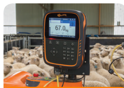
Sheep being weighed and drafted on set criteria through a Sheep Auto Drafter with the TW-1 Weigh Scale.
