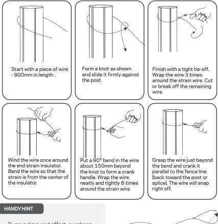
To save time and effort, purchase a Gallagher Termination Kit. This kit includes pre-assembled insulated wire strainer and wire loops for your end posts, eliminating the need for special tools or wire tying.
