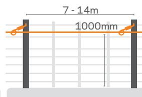
**Retrofit electric fencing** is an economical and easy to install option if you have an existing or new non-electric fence that you want to protect.
