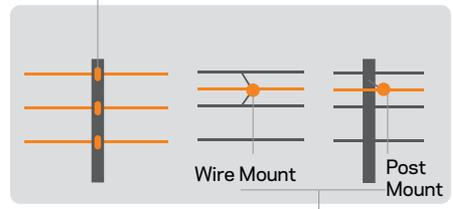
**Offsets** specific to Retrofit Fencing, hold the electric wire off the existing non-electric fence wire or posts on a conventional fence line.
